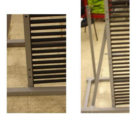
5. When both uprights are attached to the base frame and the back support braces, attach the upright support braces to the uprights using the supplied hardware.
