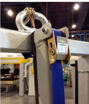
PROPER SECUREMENT OF HOLD DOWN BARS
